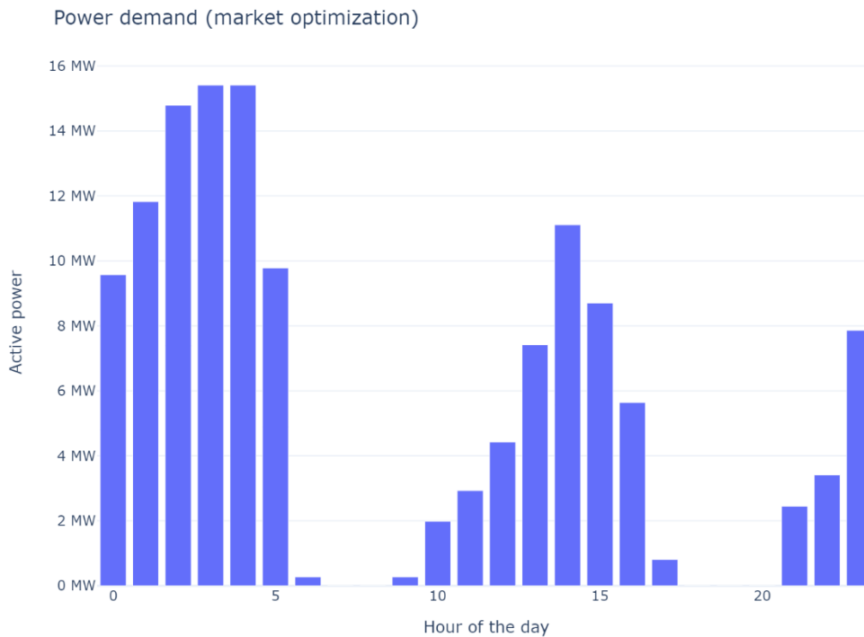
Figure 50: Power demand when optimizing 60 mixed-air compressors and fountain pumps on the day-ahead market
